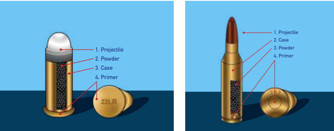
Rimfire and centre-fire ammunition.
