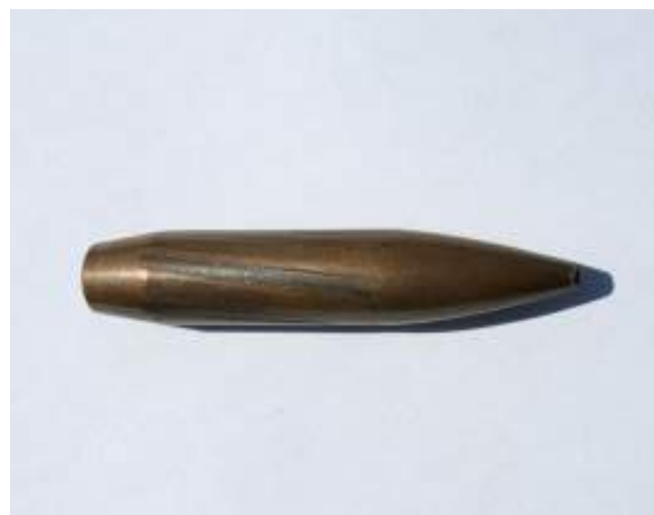
Rifling marks left on a projectile.
